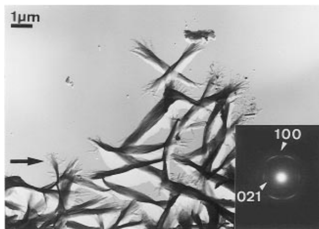
Figure 6. Sheaves of polyamide P6DM(D-L)T grown in 2-methyl-2,4-pentanediol at 80 °C. Inset: Electron diffraction from the indicated structure.
